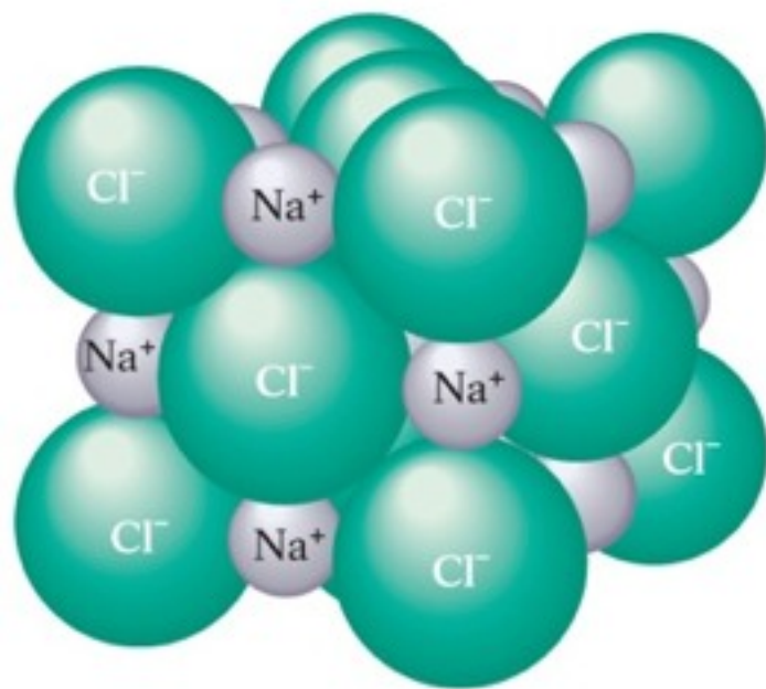
(a) Crystalline structure of NaCl
